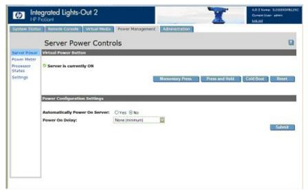
The Virtual Power Button section displays the current power state of the server as well as remote server power control options. The displayed power state is the state of the server power when the page is first opened. The server can be On, Off, or Reset. Use the browser refresh feature to keep the status of the power indicator current.
