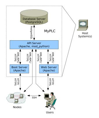
MyPLC should be viewed as a single application that provides multiple functions and can run on any host system.
